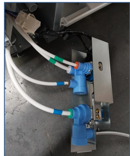
3. Pull out the water pipes on the water valve one by one
