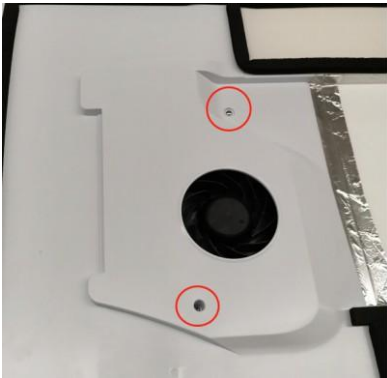
4. Remove the fan cover fixing screws
