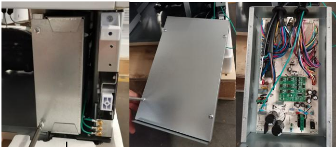
Control board repair from the lower right of the front
