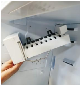
1. Take out the ice machine and remove the slides on both sides
