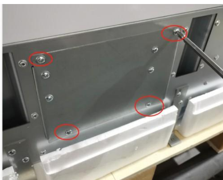
1. Remove the four screws securing the water valve from the side
