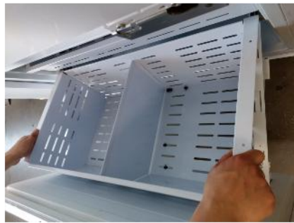
1. Pull out the freezer door body and remove the 4 handscrews
