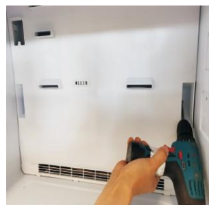
2. Remove the air duct fixing screws
