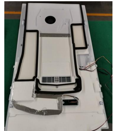
3. Remove the air duct coverplate
