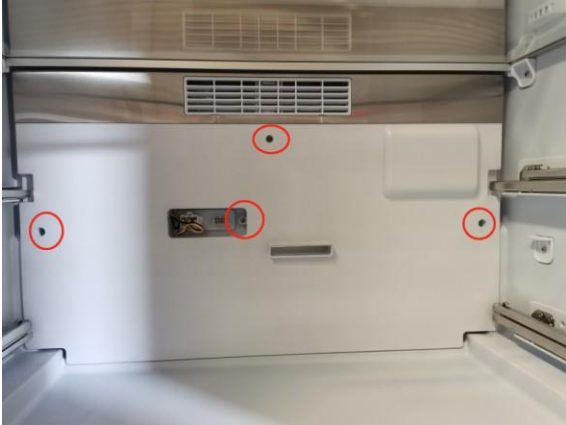
1. Remove the cover plate fixing screws
