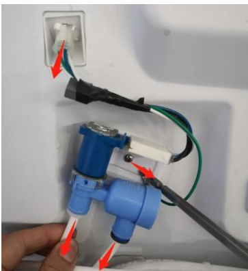
1. Remove the fixing screws and water pipes
