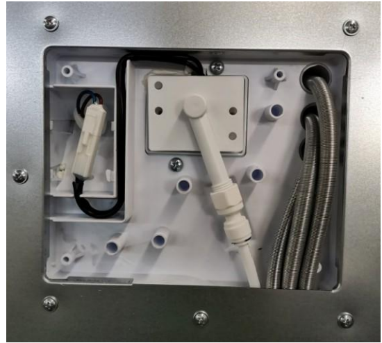
Fill Tube Heaters & Water Lines
