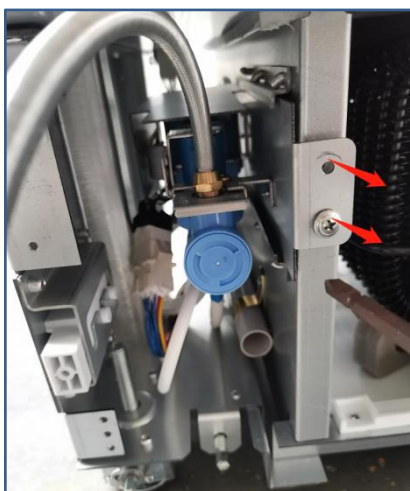
1. Remove the four screws securing the water valve from the front
