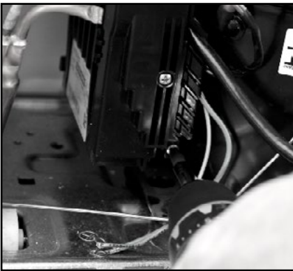
4. Remove the screw securing the inverter to the side of the compressor.
