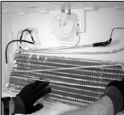
5. Carefully peel the defrost element off of the front of the evaporator.
