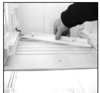
4. Remove the hose & harness cover.
