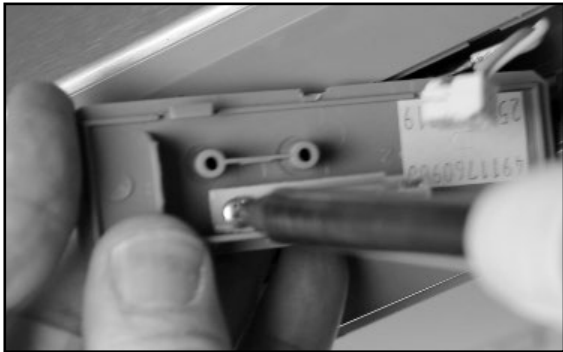
7. Unscrew the Reed Switch to remove it from the bottom access panel.
