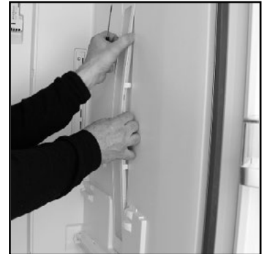
3. Unclip the side lens from the side wall.
