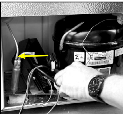
7. Using a pry tool, pull the plug and ground wire from the compressor. Note the orientation of the plug before removing.
