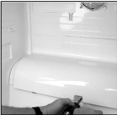
4. Remove the single screw securing the evaporator cover.
