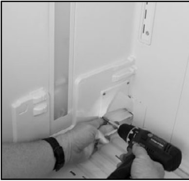
1. After removing the lower shelves and drawers, remove the three screws securing the connection cover in the left-hand side.
