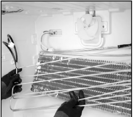
6. Peel the defrost off the back and remove. Replace in reverse order.
