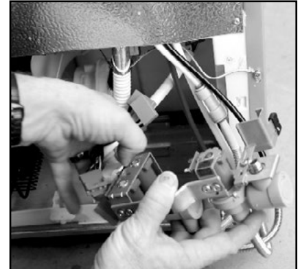
3. Unplug the harnesses from the water valve.
