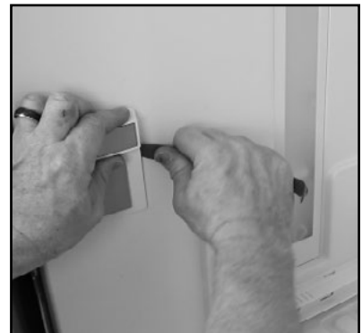
3. Carefully pry the dispenser trim from the side wall with a plastic tool.
