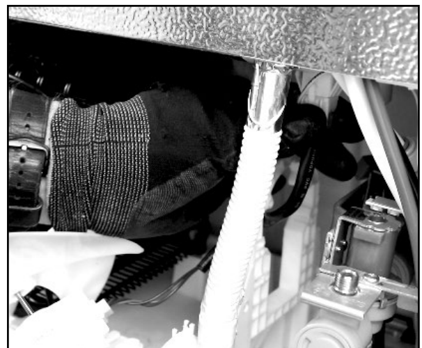
2. Unplug the fan harness from the cabinet and remove the fan. Replace in reverse order.
