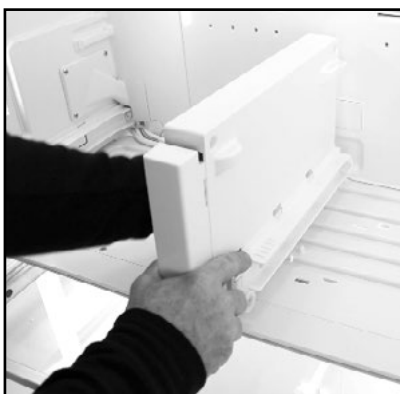
5. Lift up and pull forward on the partition. Set it off to the left side.
