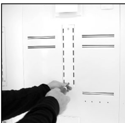
8. Remove the two T-20 Torx screws securing the middle bracket.
