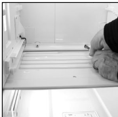
3. Remove the two screws that secure the hose & harness cover.
