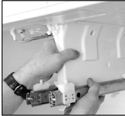
2. Remove the partition by pulling down and out.
