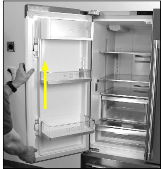
2. Lift up on the flapper heater assembly to disengage it from the door.
