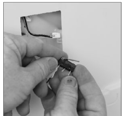
6. Unclip and unplug the microswitch to remove it.
