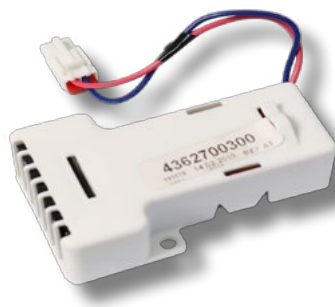
1. After removing the back panel, unplug the Ionizer, located in the upper right-hand corner.
