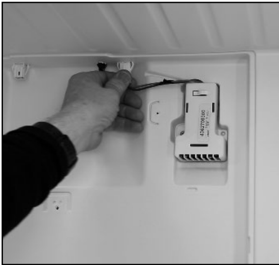
1. After removing the back panel, unplug the Ionizer, located in the upper right-hand corner.
