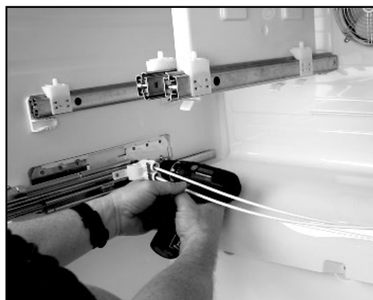
5. Using a T-20 Torx bit, remove the 9 screws securing the rails on both sides.
