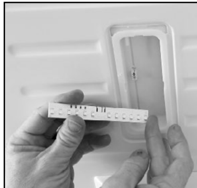
2. Unclip the light board to remove it.
