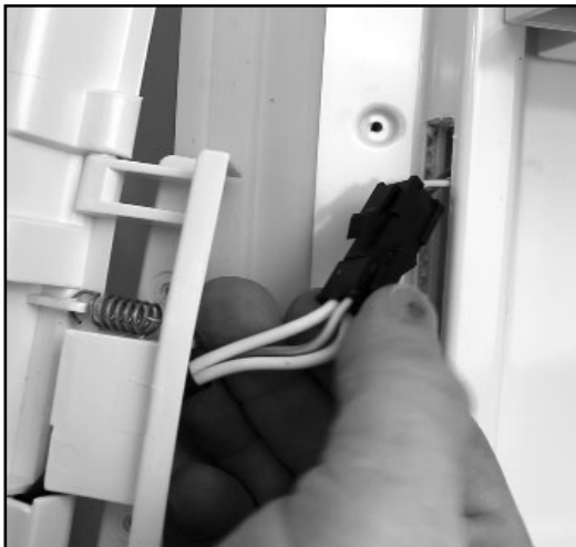
3. Unplug the flapper heater harness to remove the heater.
