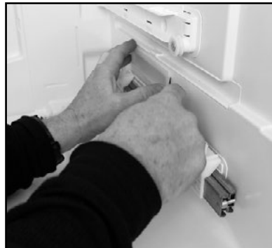
5. Unclip the bottom lens to access the light board.
