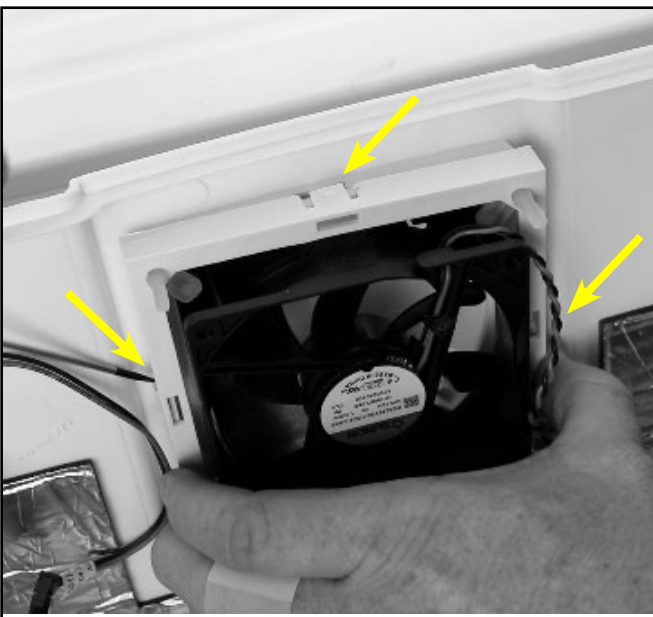
1. After removing the rear panel, unclip the four retaining clips on the fan trim. Note: Be sure to note the direction of the fan, as indicated by the sticker on the fan hub. Replace in the same direction.
