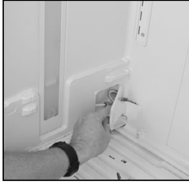
2. Disconnect the water line to the dispenser from the John Guest fitting.
