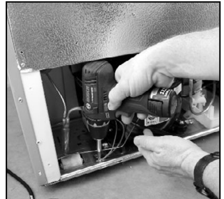
3. Remove the screw securing the ground wire.
