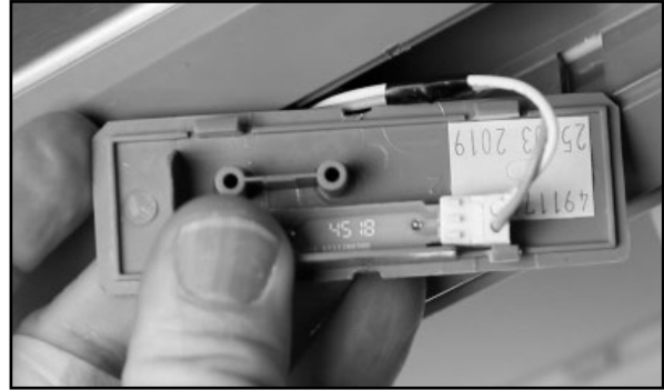
6. Unplug the harness to the Reed Switch.
