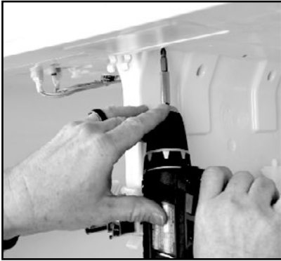
1. Remove the four screws securing the partition to the Freezer ceiling.
