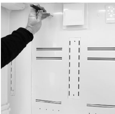
9. Carefully remove the two screw covers at the top of the rear panel.
