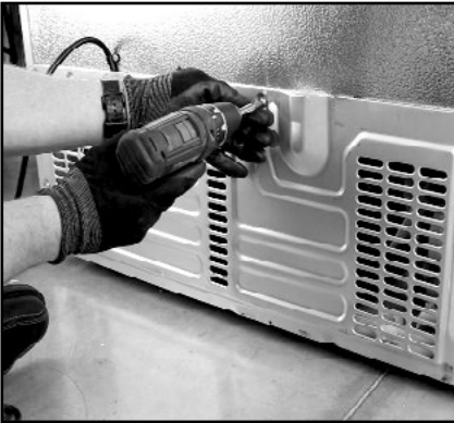
1. Remove the six screws securing the compressor.
