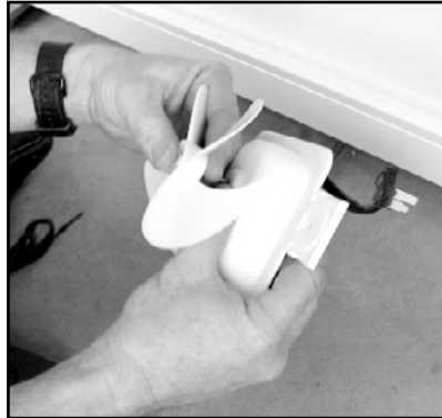
8. Pull the fan blade from the shaft.
