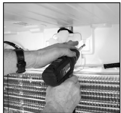
6. Remove the two screws securing the fan to the rear wall.
