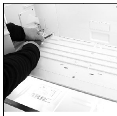
6. Remove the single screw securing the bottom shelf.
