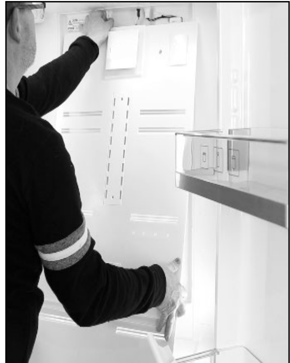
12. Unplug the Fan and Light harnesses and remove the rear panel.
