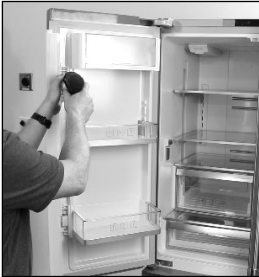
1. Remove the four screws securing the flapper heater to the door.
